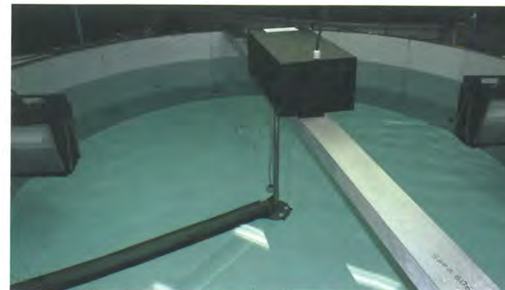
Self cleaning tank with arm and outlet filters.
